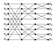
• At stage *m* of algorithm, tasks *k* and *j* exchange data, where *k* and *j* differ only in their *m*th bits
